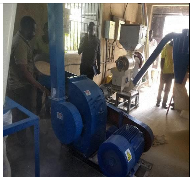
Maize milling equipment installed under NAADS intervention being inspected and test run at beneficiary sites in Bugiri and Mayuge Districts.
