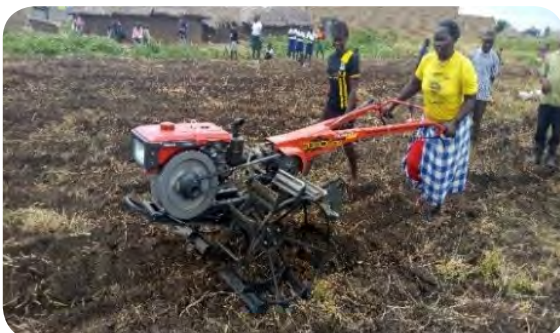
Power Tiller (walking tractor)
