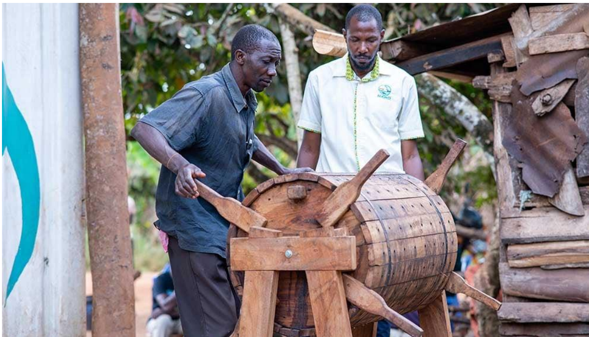
Figure 26: NaCORI single-box cocoa fermentation system.
