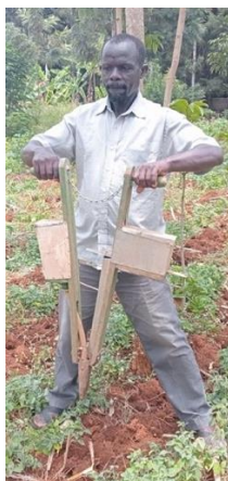
Figure 11: The planter has both the seed and fertilizer boxes
